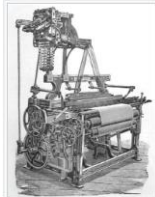
A loom from the 1890s with a dobby head. Illustration from the Textile Mercury.
